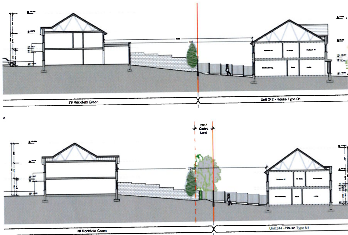
Figure 3.11: Section with 29 and 30 Rockfield Green
